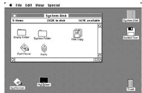
On the top left of the screen, anchored by an apple, the nested pull-down menus performed system-wide actions. Here is the Macintosh control panel [↵], a tour de force of early interface design.
